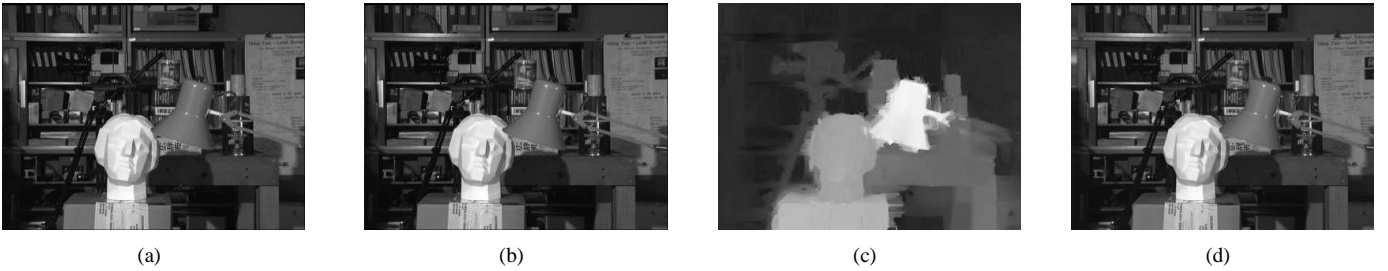
Fig. 7. Recovery of depth information from a stereoscopic image pair using the ROF model. (a) Left image. (b) Right image. (c) Disparity field after optimization. (d) Warped right image.
