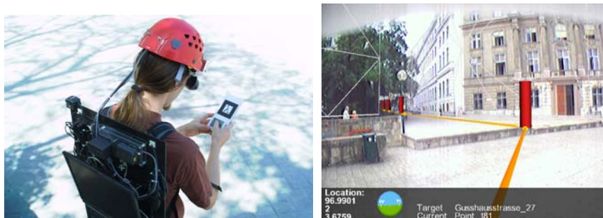
Figure 2 (Left) User interacting with a mobile AR system, (Right) Outdoor navigation display leading a user down a street
