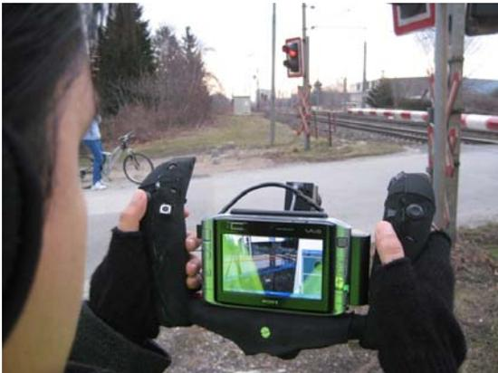
Fig. 1: VIDENTE handheld augmented reality client platform
